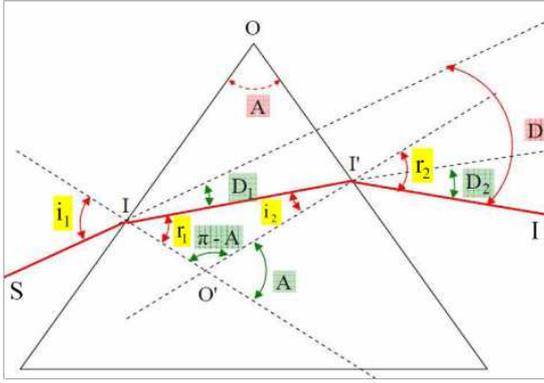
$$\begin{aligned} \sin i_1 &= n \sin r_1 \\ n \sin i_2 &= \sin r_2 \\ r_1 + i_2 &= A \\ D &= i_1 + r_2 - A \end{aligned}$$
